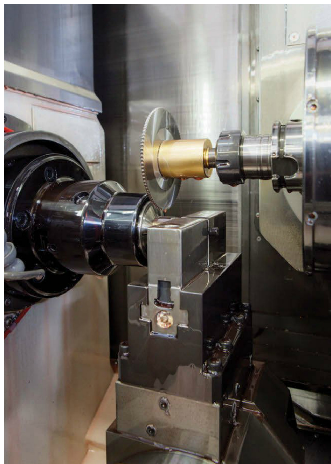
Lowell's Integrex i-150 features a C-axis CNC-controlled turning spindle, vertical B-axis milling spindle and back working vise/part support center.
